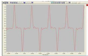
Strain Data obtained from Strain Gage Amplifier (US Manufacturer). Cost Per Channel $4K+
