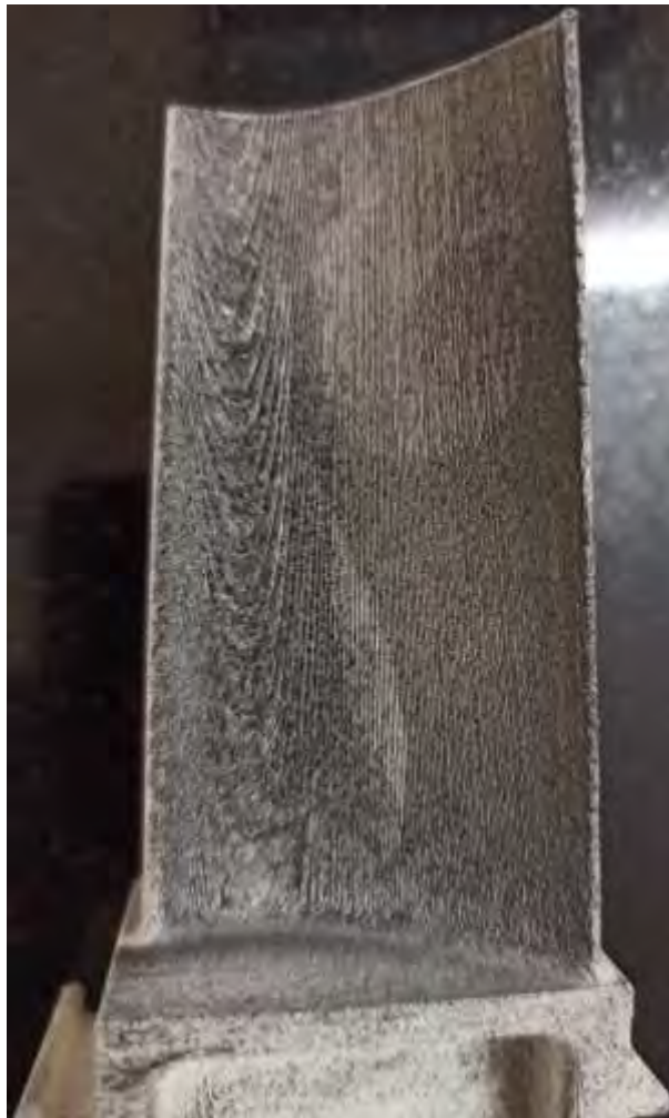
Speckle pattern applied on the Gas Turbine Blade using an Air Brush.
