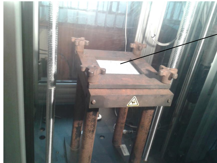
Plunger striking the specimen (Image captured by the camera)
