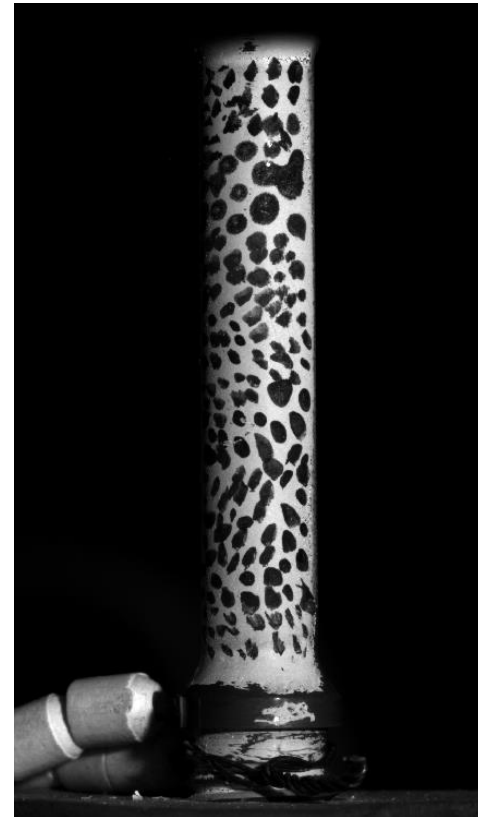
Speckle Image at Elevated Temp – 800 Deg C
