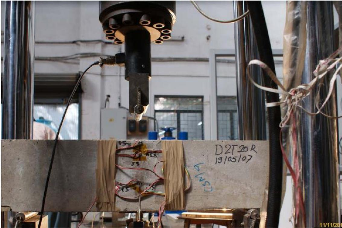
A speckle pattern was applied on the concrete Beam with a notch under test.
