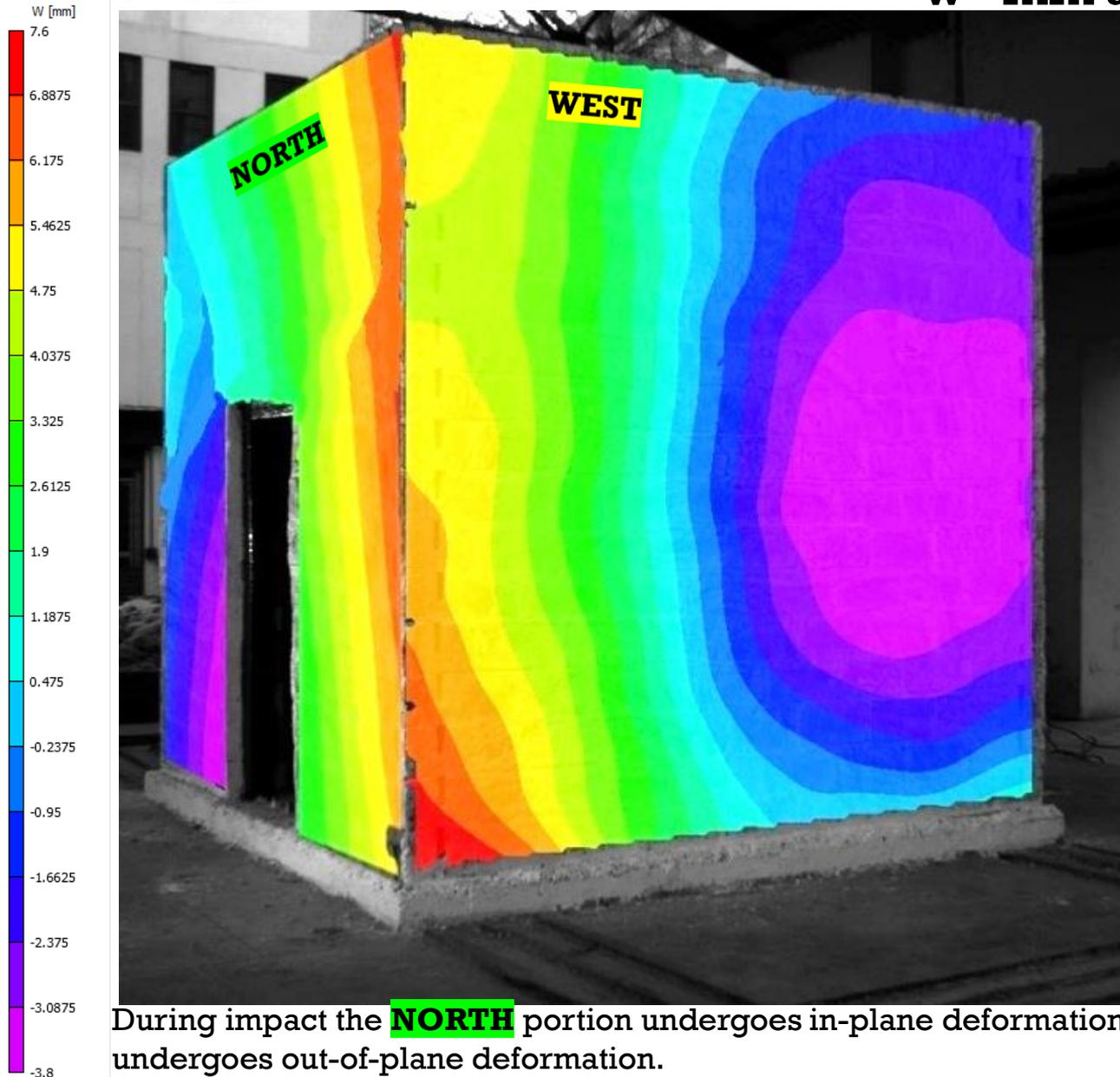
During impact the **NORTH** portion undergoes in-plane deformation and **WEST** portion undergoes out-of-plane deformation.
