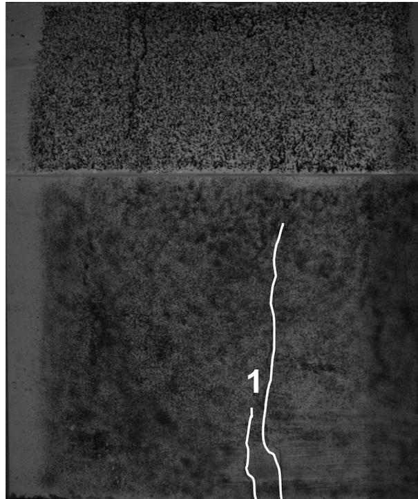
Image no 553 - just after the load crossed phase 7- Specimen cracked at this Load.
