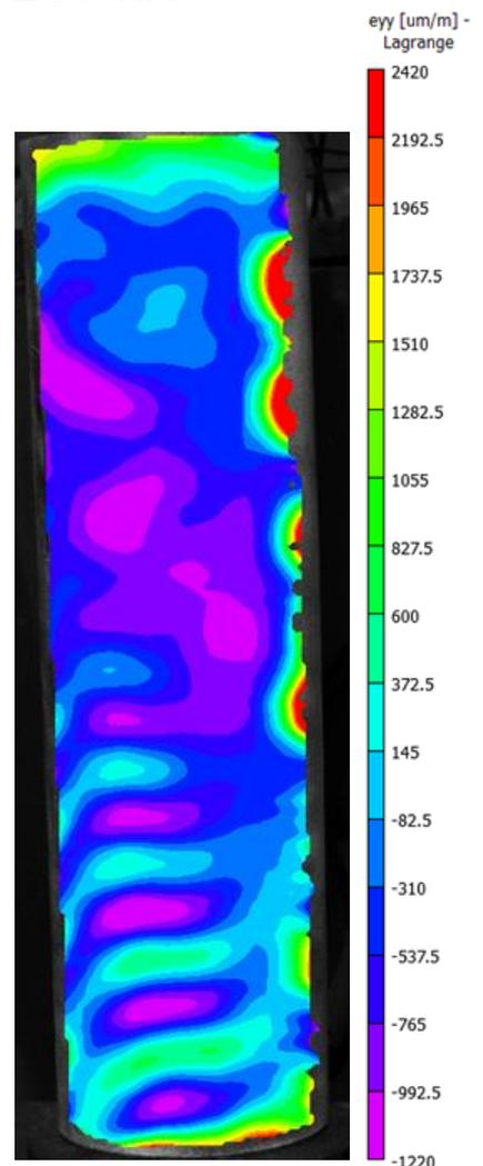
**Strain Plot just before complete failure**
