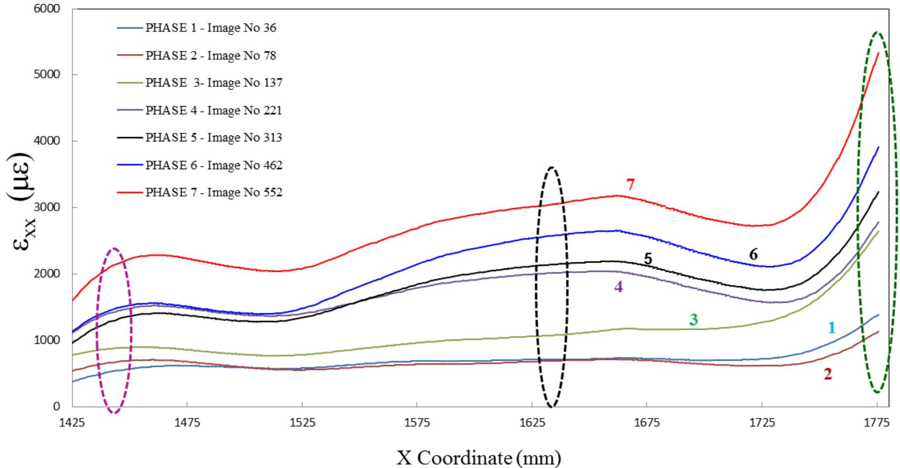
Very Good Linearity observed in the strain field at Peak Loads of Different Phases of Loading.
