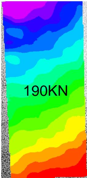
Since the concrete beam under load has a downward displacement the DIC shows a negative value.
