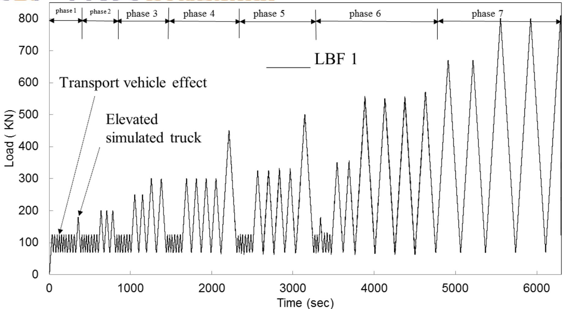
❑ Crack observed in the Sixth Phase at peak load of 670 kN.
