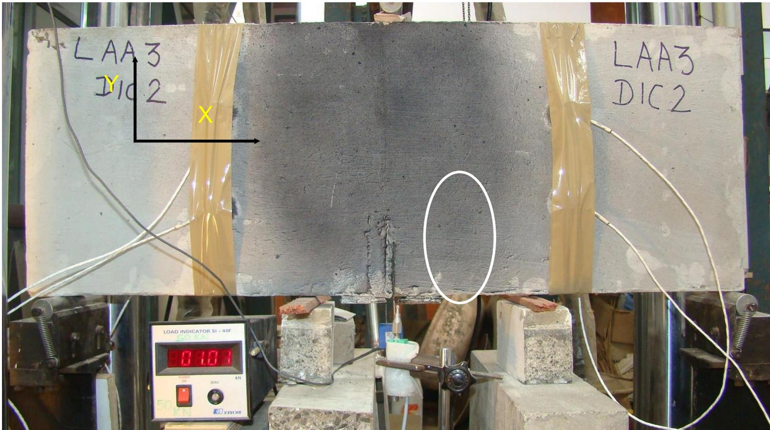
Under load the crack opens in the X Direction
