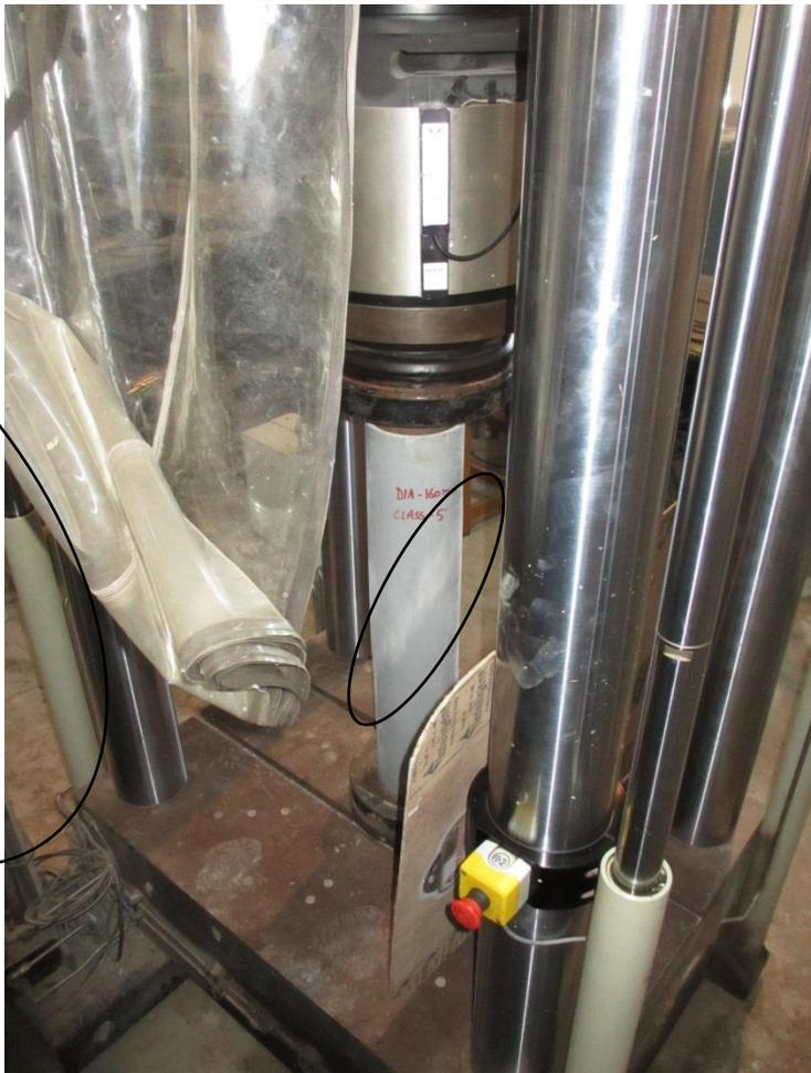
The concrete column had a shear crack and failed at 1260 kN.
