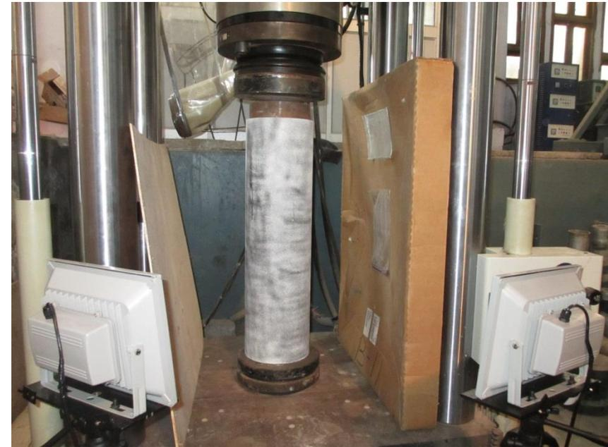
A concrete column – 600mm long, 225mm Diameter was wrapped with a 7mm thick PVC sheet.
