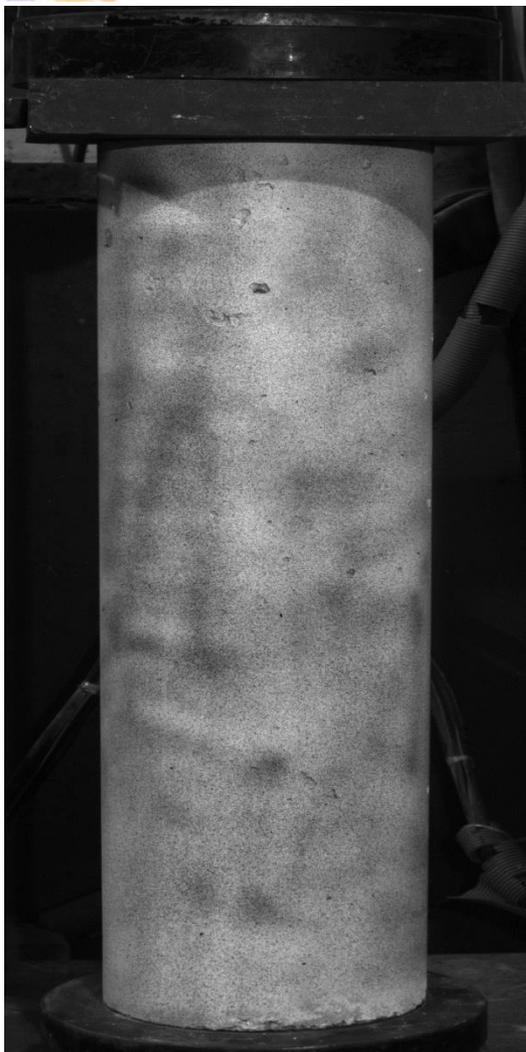
Compressive Load was applied on a Concrete Column 800 mm Long , 218mm Diameter.
